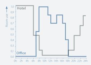
Offices are mainly used during the day whereas hotels are mostly used in the early morning and in the evening. Cross-floor room automation makes it possible to exploit all energy saving potential on the basis of an accurate use profile that depends on requirements and the presence of people.
